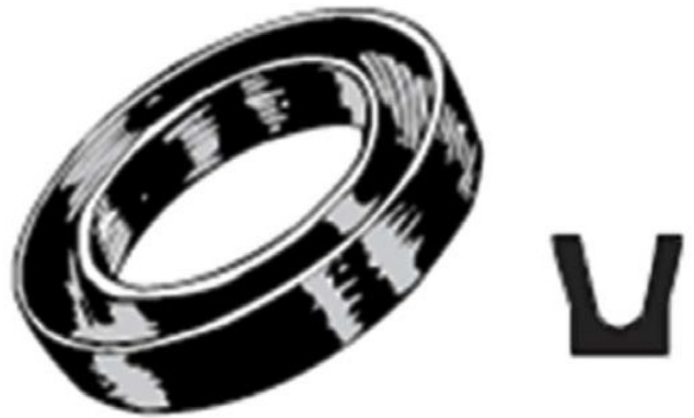
Figure 7-22 — Typical U-cup seal.
